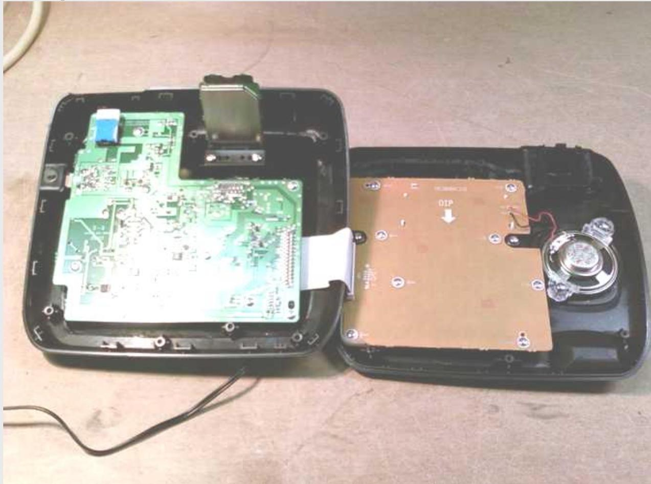
Uniden TRU-9488 Base Unit - lid folded back. RF Module is standing up vertical in the main circuit board cutout. There is space for a Type N External Antenna connector to the right of the RF Module.
