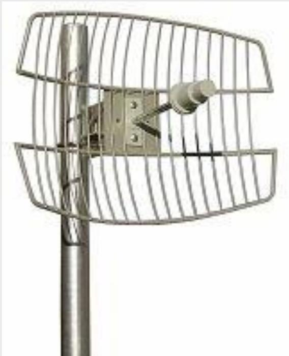
Pacific Wireless Inc Grid 58-22 Para-Grid Antenna. 21/22 dBi. 10° Beam Width. Weight 8 lbs. Welded steel rods, galvanized and powder coat painted. Low wind loading. Bulkhead N Female connector. US\$55 (US\$3 less than the 27dBi model approved for purchase.
