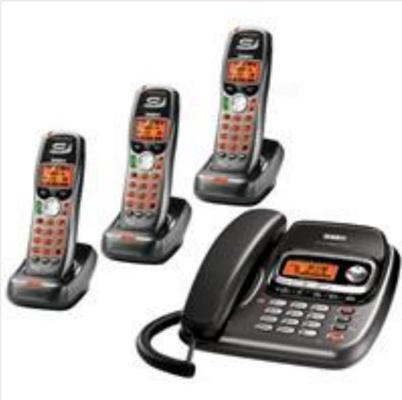
*This Uniden model uses frequency-hopping digital spread spectrum mode. Most cheaper models are analog FM and operate base-handset at 5.9GHz but handset-base at 900 MHz. The corded handset in this base replaces the P.O.T.S. for speech to/from handsets.*
